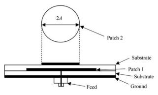
Fig. 2. Cross-sectional view of single-feed stacked microstrip antenna.
