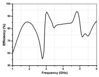
Fig. 13. Variation of simulated radiation efficiency (%) with frequency (GHz) for circularly polarized stacked microstrip antenna.
