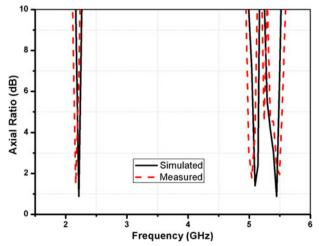
Fig. 11. Variation of axial ratio (dB) with frequency (GHz) for circularly polarized stacked microstrip antenna.
