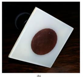
Fig. 3. Prototype of the fabricated antennas (a) compact circularly polarized square microstrip patch (b) circularly polarized stacked microstrip structure.
