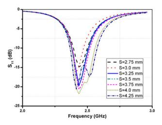
Fig. 4. Variation of  $S_{11}$  (dB) with frequency (GHz) for different S without circular slot loaded in the center.
