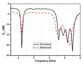
Fig. 10. Variation of  $S_{11}$  (dB) with frequency (GHz) for circularly polarized stacked microstrip antenna.
