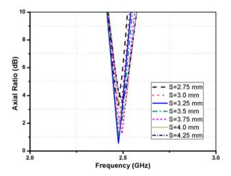
**Fig. 5.** Variation of axial ratio (dB) with frequency (GHz) for different *S* without circular slot loaded in the center.
