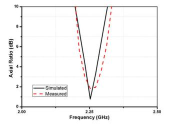
Fig. 7. Variation of axial ratio (dB) with frequency (GHz) for circularly polarized circular slot loaded square microstrip antenna.
